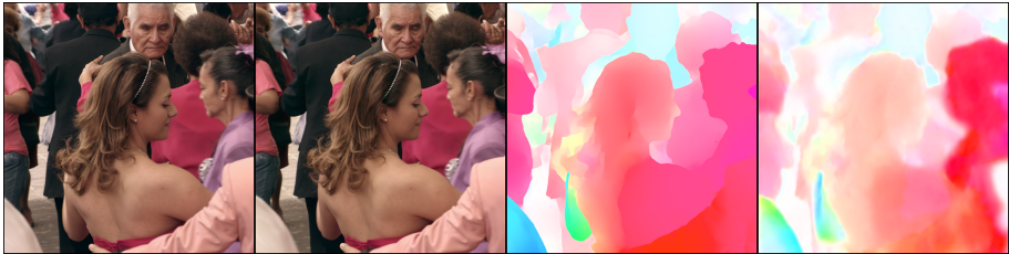
Fig. 7. An example of the estimated optical flow, left to right: two consecutive frames used for estimation, FlowNet2 results, our decoder output \hat{\mathbf{f}} . Note that the flow produced by our model is decoded from a compressed latent, and is trained to maximize total compression performance rather than warping accuracy. See Appendix B for license information.
