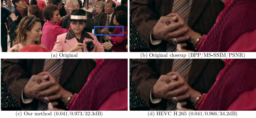
Fig. 6. An illustration of qualitative characteristics of our architecture versus H.265 ( ffmpeg ) at a comparable bitrate. (a) and (b) are the original frame and its closeup, (c) and (d) are the closeup on the reconstructed frames from our method and H.265. To make the comparison fair, we used HEVC with fixed GoP setting ( min-keyint=8:scenecut=0 ) at a similar rate, so both methods are at equal bpp and show the 4th P-frame of a GoP of 8. Frame 229 of Tango video from Netflix Tango in Netflix El Fuente; see Appendix B for license information.
