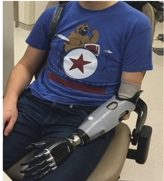
Fig. 39.33 Myoelectric prosthetic after elective amputation
