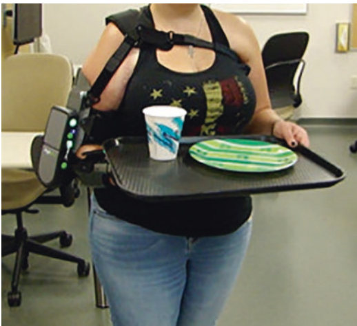
Fig. 39.32 MyoPro use with bilateral hand function: carrying a tray
