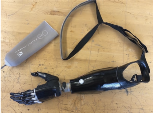
Fig. 38.1 Transradial prosthesis with flexible supracondylar cuff, figure-9 harness with linear transducer excursion. Silicone liner with pin suspension. Manual flexion-extension wrist. Externally powered terminal device
