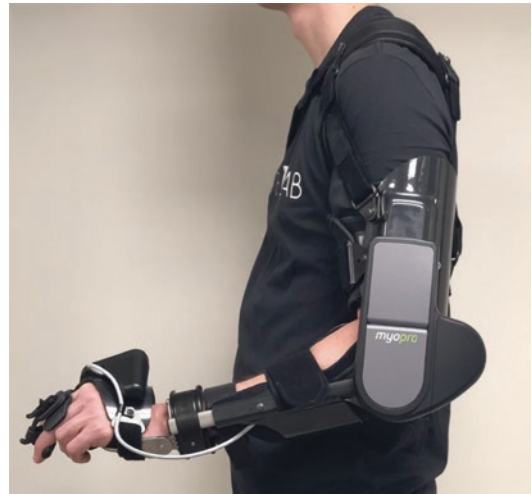
Fig. 38.7 The MyoPro Motion G custom-fabricated myoelectric orthosis. The electrodes are housed within the humeral cuff and forearm cuff, reading the muscle signals from the biceps, triceps, wrist flexors, and wrist extensors. The multi-articulating wrist allows for passive pronation, supination, wrist flexion, and wrist extension. Velcro closures are applied at the hand, forearm section, humeral section, chest strap, and axilla saddle. Donning begins distally at the hand and moves proximal, working one joint segment at a time to assure proper positioning and alignment
