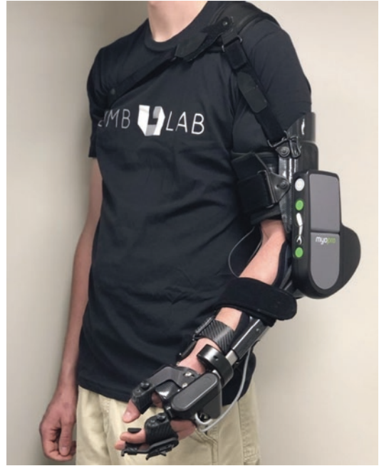
Fig. 38.8 The MyoPro Motion G, incorporating a three-jaw chuck grasp with multi-articulating wrist. The battery source is located on the lateral portion of the device. The various modes to the elbow and hand can be readily accessed by clicking the green buttons. Mode options include elbow only, hand only, or both elbow and hand. Electrodes need to make direct contact to the skin for accurate detection of the muscle signal. The gain, boost, and threshold settings can be adjusted within the software for consistent, reproducible outputs that will restore physiological elbow and hand motion
