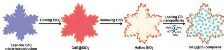
Scheme 3.7 Illustration for the preparation of the SiO 2 @CS composite with a biomimetic leaf-like structure. (Liu et al. 2019)
