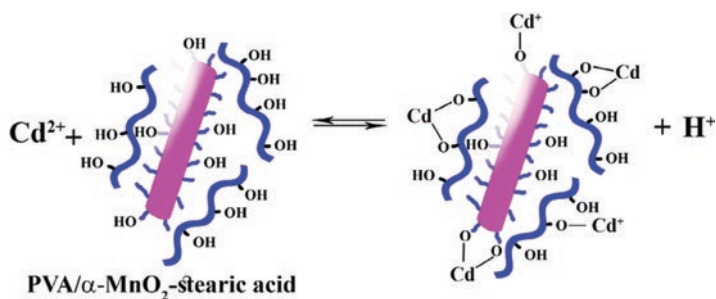
Scheme 3.8 The mechanism of \text{Cd}^{2+} ion adsorption onto PVA/ \alpha\text{-MnO}_2 -stearic acid NC. (Mallakpour and Motirasoul 2017b).
