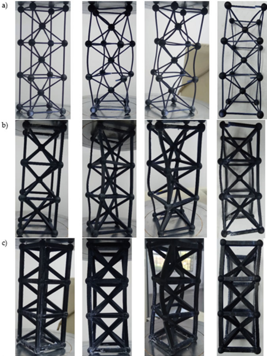
Fig. 11 Deflections and cracks in a 2, b 4, and c 6 mm of MJP samples
