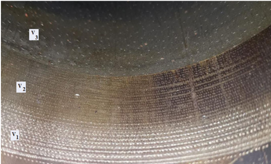
Fig. 8 Percussion dispersion depending on the speed and advance of the device
