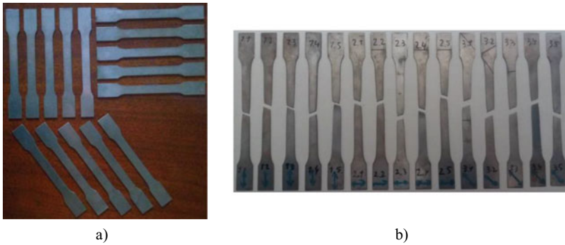
Fig. 7 Tensile test: a specimens on the cutting directions, b tested specimens [5, 18]
