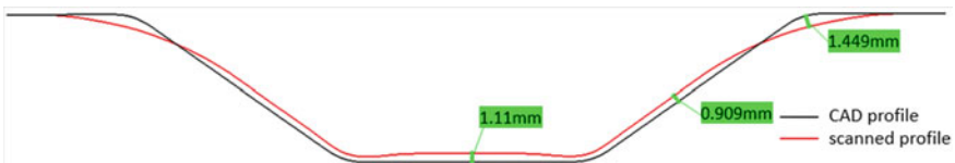
Fig. 26 Dimensional precision for CONE-D85H20 \alpha 35 \Delta z0.5 part [5]
