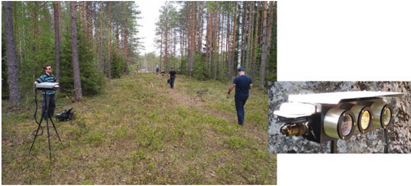
Fig. 16.2 The SMARTSENSE platform (battery driven and mountable on trees or masts)
