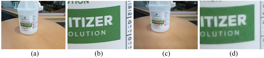
Fig. 1. Images taken under different ISO settings. (a) ISO100, (b) magnified region of (a), (c) ISO3200, (d) magnified region of (c).
