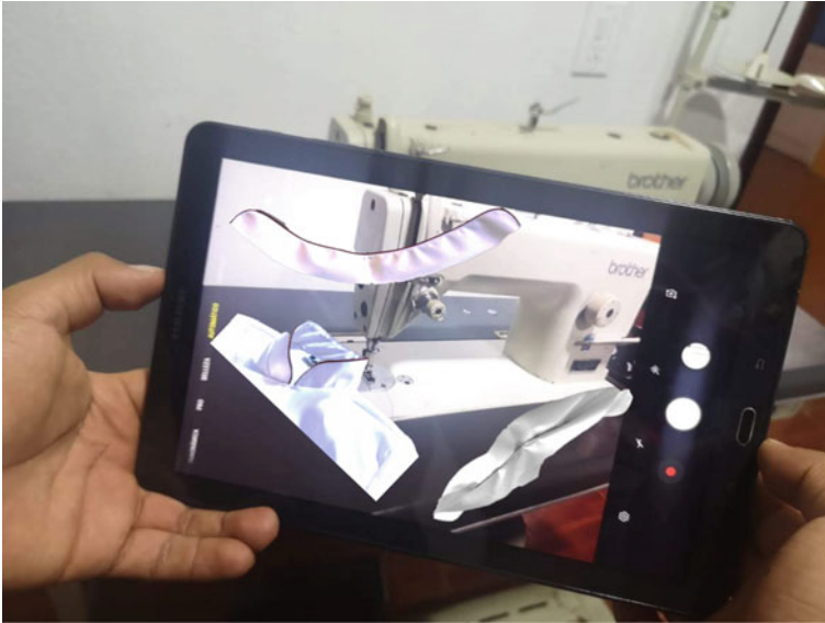
Fig. 4 Assembly parts for the collar of a Balloon Shirt using the AR
