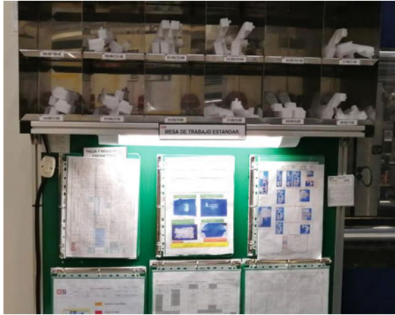
Fig. 10 Special containers for hour-by-hour inspection
