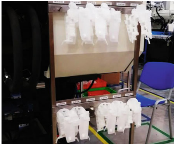
Fig. 11 Special containers for hour-by-hour inspection
