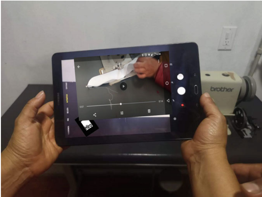
Fig. 6 AR system, showing the assembly process by means of a video
