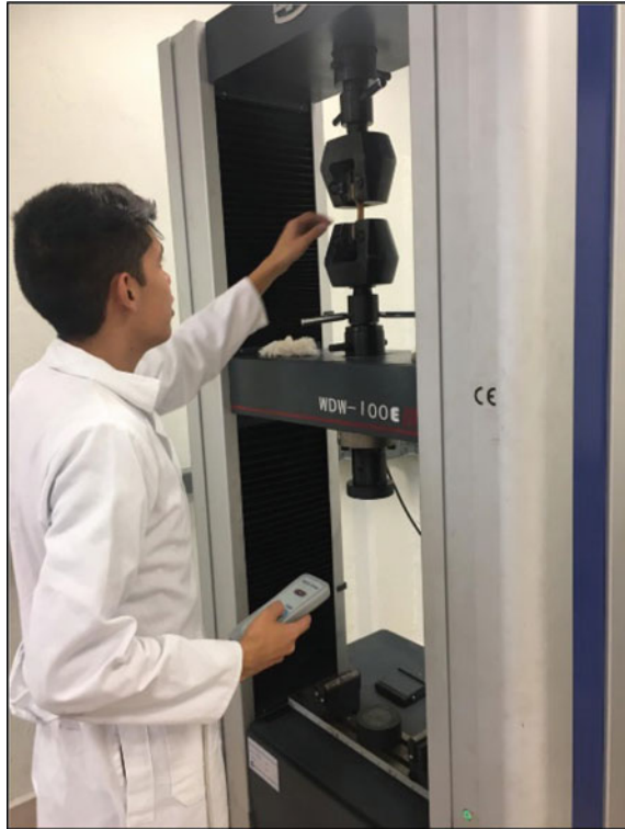
Fig. 2 Tensile tests performed on the universal machine
