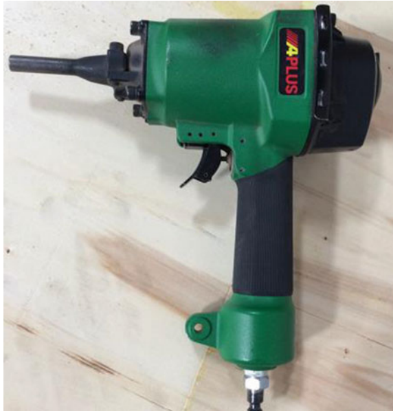
Fig. 12 Air gun implemented in the process of disassembling
