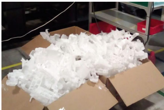
Fig. 3 Produced scrap by a wrong defect identification on production pieces
