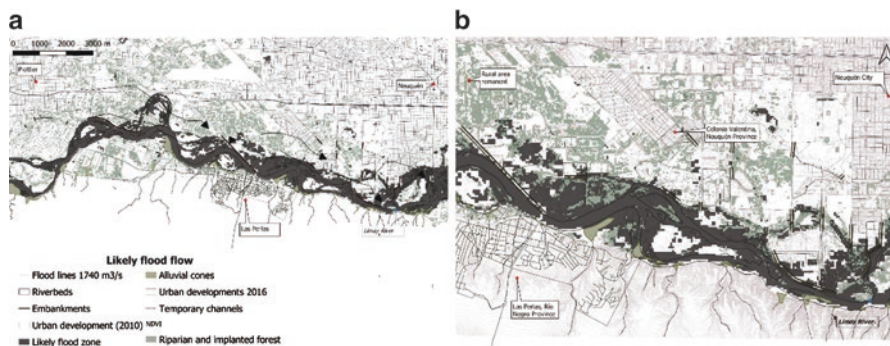
Fig. 17.2 (a) Flood risk map of the Limay river for a recurrence flow of 14 years ( Q = 1740 \text{ m}^3/\text{s} ). (b) Possible channels for channeling a flood ( Q = 1740 \text{ m}^3/\text{s} ) in an area occupied by embankments, artificial slopes, and elevated streets
