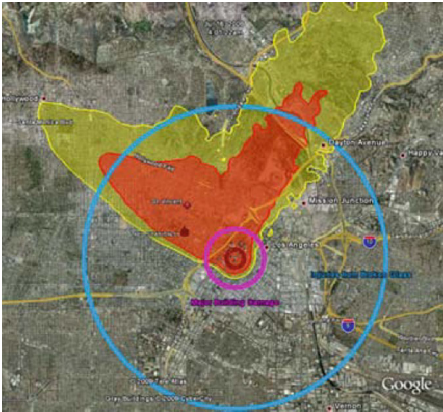
Fig. 10.2 Map of fallout (orange and yellow) and blast effects from a simulated 10 kt attack. Note the bifurcated plume, due to upper-level and lower-level winds blowing in different directions [5]
