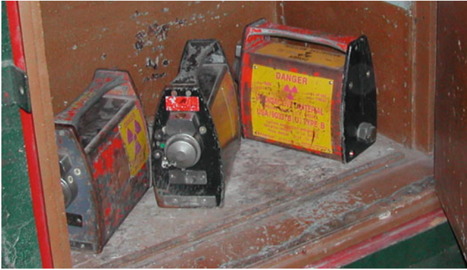
Fig. 14.2 Three older-style industrial radiography “cameras.” Each of these is a lead or depleted uranium radiation shield containing a radioactive source of a few TBq in activity. (Author’s photo)
