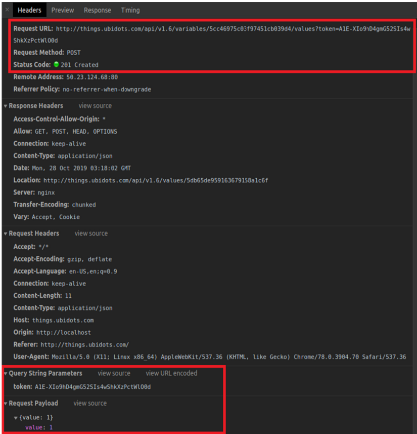
Fig. 11. Request with signal to turn on “led9” variable.
