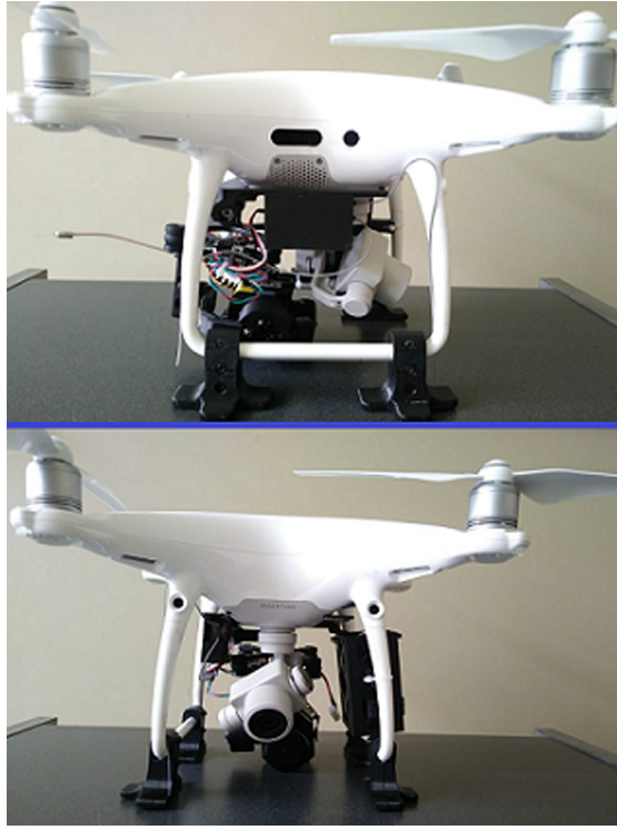
Fig. 5. Drone with RGB and thermal camera used in this research.
