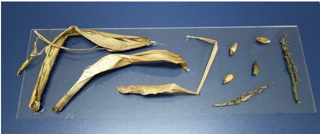
Fig. 8. Glass with dry leaves and seeds to simulate dirt obstructing the radiation path in three PV cells.
