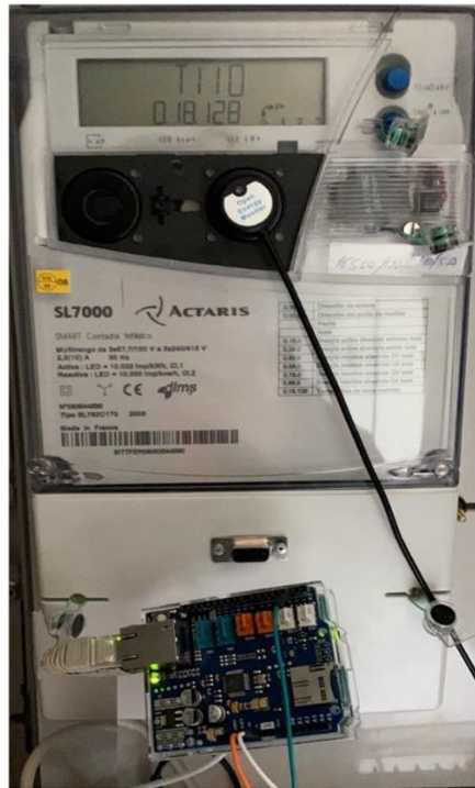
Fig. 4. Mounting the measuring system on the counter.
