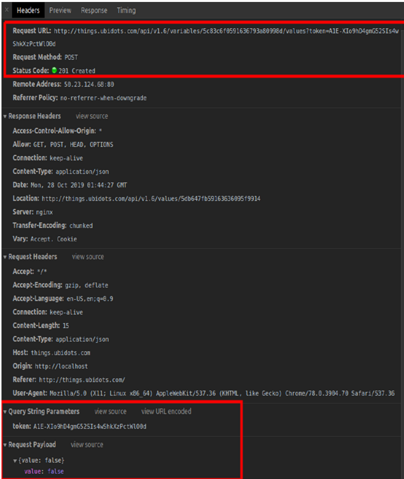
Fig. 10. Request with signal to turn off “led1” variable.
