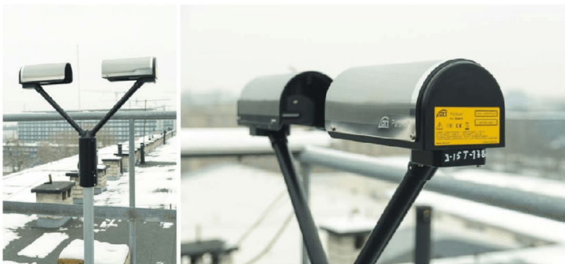
Fig. 4. OTT Parsival2 laser disdrometer ( https://www.ott.com/products/meteorological-sensors-26/ott-parsival2-laser-weather-sensor-2392/ ).
