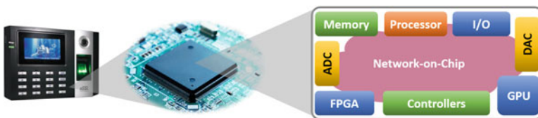
Fig. 1.1 An example System-on-Chip (SoC) with Network-on-Chip (NoC) based communication fabric to interact with a wide variety of third-party Intellectual Property (IP) cores
