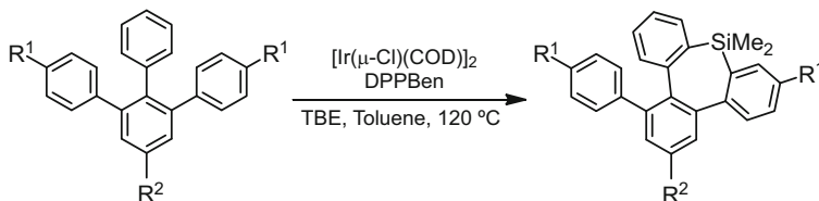
Scheme 38 Catalytic preparation of tribenzosilepins by dehydrogenative silylation
