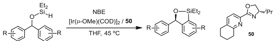
Scheme 29 Silylation of symmetric diarylmethoxy diethylsilanes with chiral pyridinyloxazoline ligand 50
