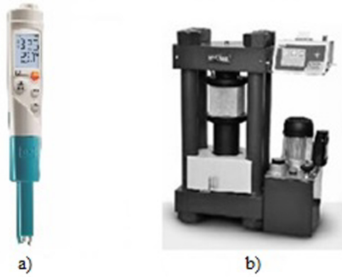
Fig. 1. a) Portable certified pH meter by brand Testo 206 PH1; b) Testing press by brand Matest C055N.
