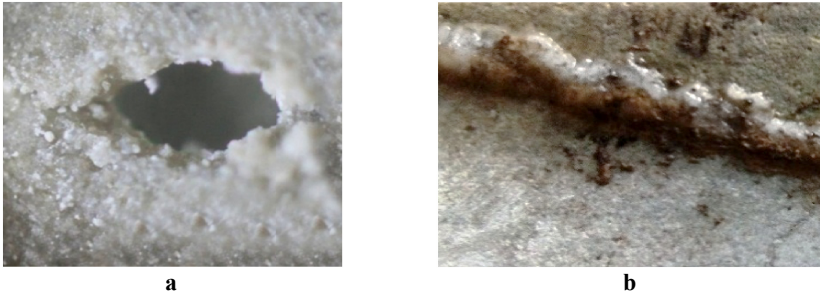
Fig. 3. a. Image (x60) of the cement stone surface in case of biodamage. b. Image of the cement stone surface in case of bio-damage in the period of 28 days.
