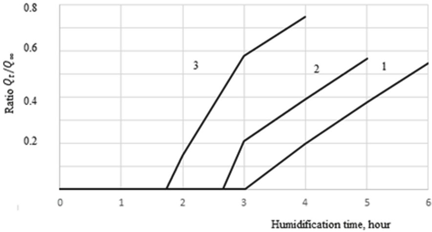
Fig. 3. Kinetics of moisture accumulation at the “coating-substrate” interface depending on the surface porosity of the substrate: 1-substrate with porosity P_p = 0\% ; 2 - substrate with porosity P_p = 0.4\% ; 3 - substrate with porosity P_p = 1.13\% .
