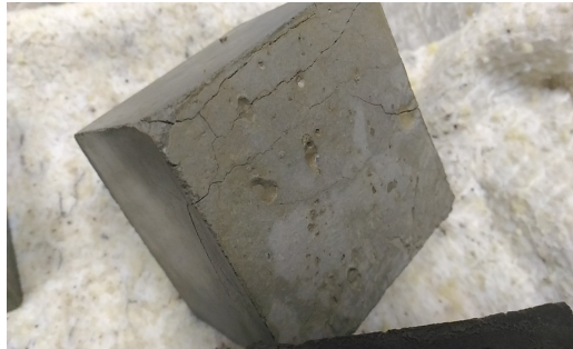
Fig. 1. Sample of compound №2 after frost resistance tests.
