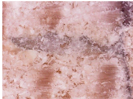
Fig. 3. Glue spreading through the pin hole.
