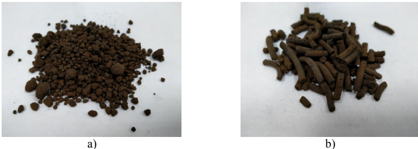
Fig. 3. Granules received a) Torsion type granulator b) Screw type granulator.
