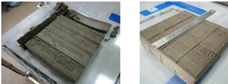
Fig. 2. Production of printed samples for determination of strength.
