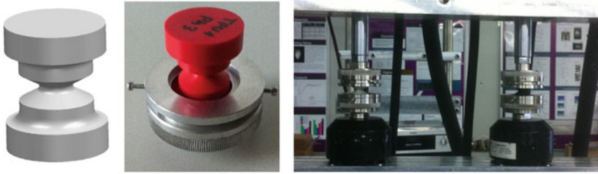
Fig. 1 Cylindrical “diabolo-type” test specimen, fixture and test setup
