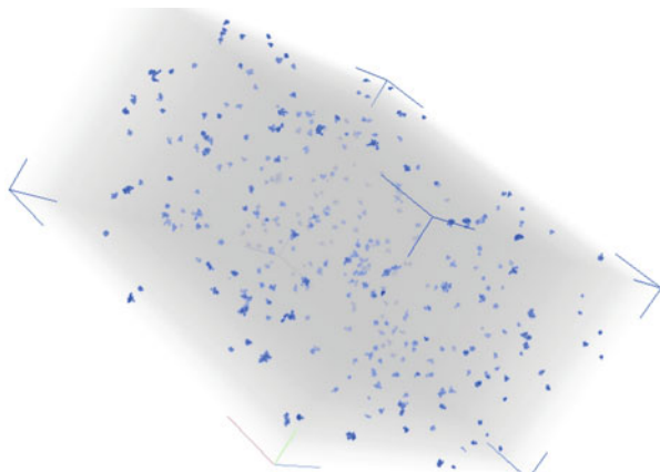
Fig. 2 Density contrast for a CT investigation reconstruction for CB filled NR material, voxel size 9\ \mu\text{m} [29]
