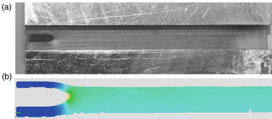
Fig. 5 (a) Notched PS test specimen of a TPU with blunted crack tip and (b) the local crack tip strain measured by digital image correlation (enlarged)
