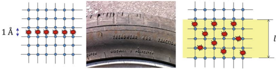
Fig. 6 Left: idealized crack with zero thickness; middle: visible closed crack in unloaded tire; right: realistic bulk crack with finite thickness l
