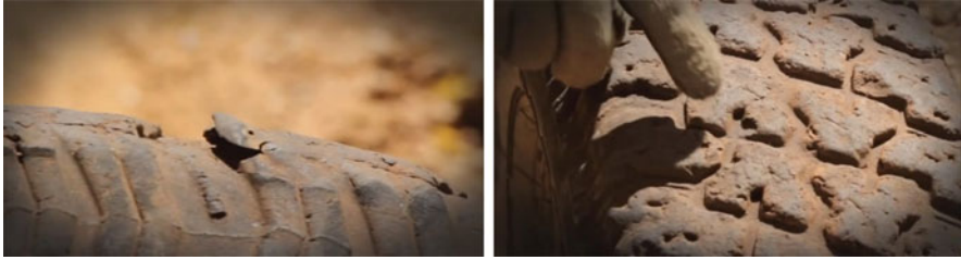
Fig. 3 Photograph of locally rupture tyre treads due to different mechanism ( https://www.youtube.com/watch?v=bTnE66fvjrl )
