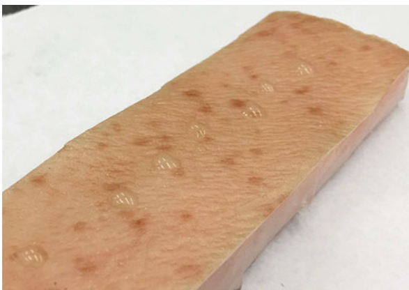
Fig. 34 After injecting the fluid and removing the needle, the fluid pressure in the cavity is high enough to allow some fluid to leak to the surface of the skin where it forms small water droplets
