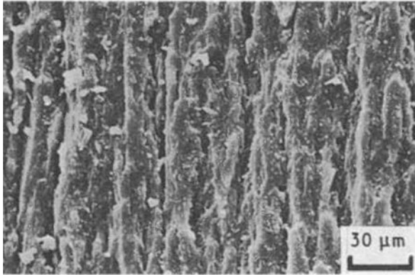
Fig. 35 Wear tracks on rubber surface
