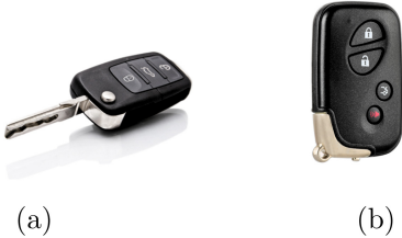
Fig. 2. Car key models: (a) RF remote controller key, (b) RFID keyfob.
