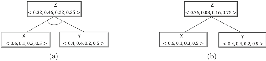
Fig. 6. Computing an opinion on event Z via (a) AND gate, and (b) OR gate.
