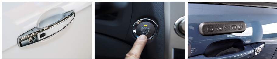
Fig. 3. RFID push button on door handle (left), the “Start Engine” button (center), and the car door-keypad used on certain American car makes such as Ford, Cadillac, Lincoln, Mercury, and Chevrolet, since the early eighties (right).
