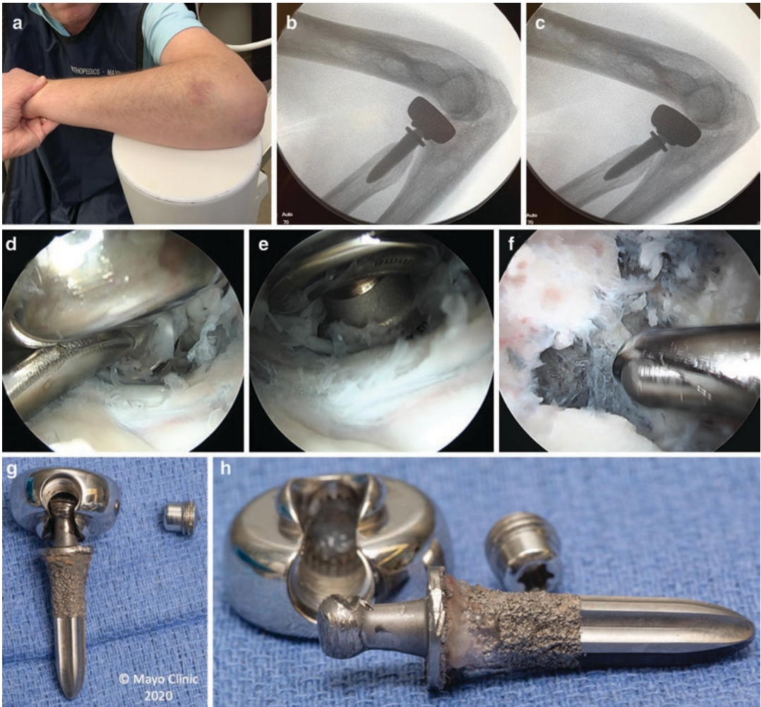
Fig. 4.21 Example of disengagement of an adjustable angle locking mechanism using a bolt. (a) Positioning the elbow for comparison lateral X-rays in flexion and hyperflexion. (b) Lateral view in flexion. (c) Hyperflexion causes the head to tilt on the neck, indicating that the locking mechanism is no longer working, but causing metal-on-metal abrasion. (d and e) Arthroscopic reviews of the
