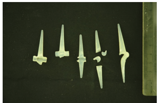
Fig. 20.16 Fracture of the silicone implant
