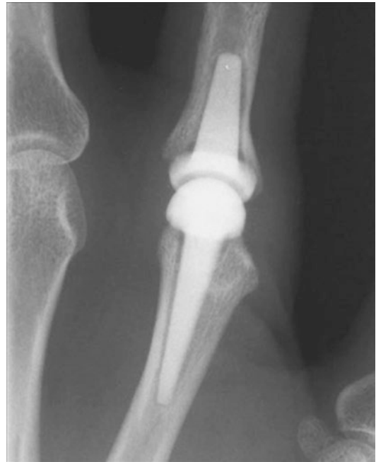
Fig. 16.10 Radiographic image of the graphite substrate and the radiolucent PyC coating
