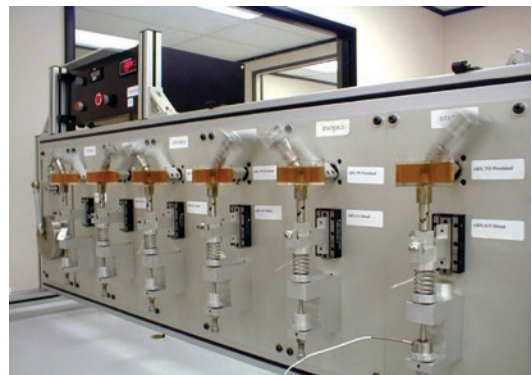
Fig. 16.12 Station MCP joint wear test machine
