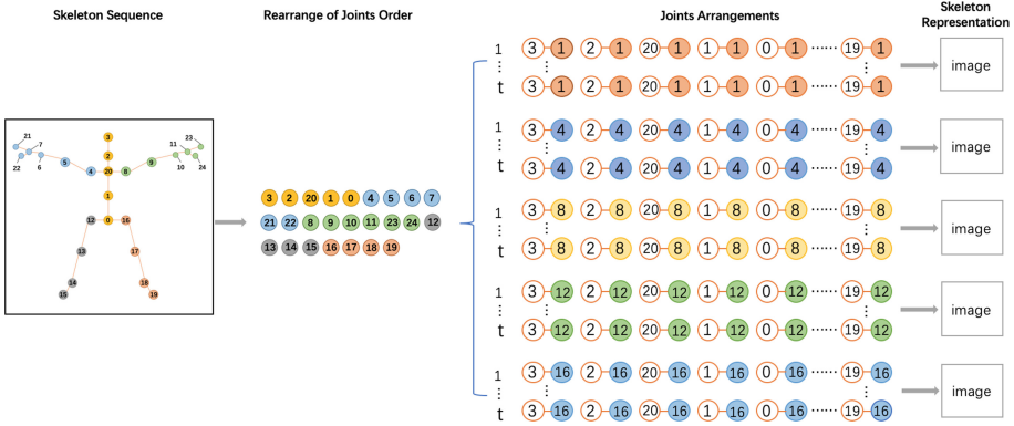
Fig. 3. The process of encoding skeleton representation from original skeleton sequence. For each input skeleton sequence, the order of the serial number of joints is first rearranged by our proposed method. Then the relative distance between key joint and other joints are calculated respectively. Each key joint corresponds to an encoded grayscale image and five images revealing the relative distance are generated.
