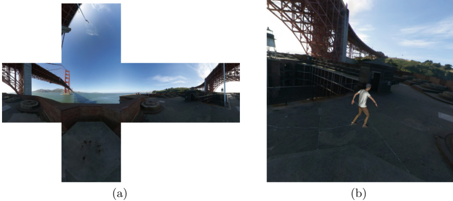
Fig. 3. (a) Example of an unfolded cube projection of a 3D environment (extracted from [1]). (b) Example of a 3D body scan added to the 3D environment of a realistic scene.
