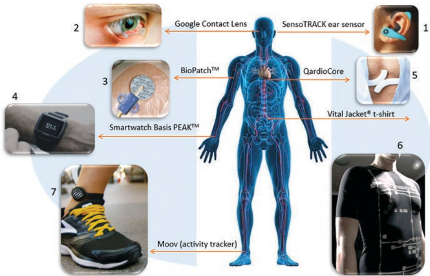
Fig. 2 Several wearable health monitoring devices, including (1) SensoTRACK ear sensor, (2) Google Contact Lens, (3) BioPatch™, (4) Smartwatch Basis PEAK™, (5) QardioCore, (6) Vital Jacket® t-shirt, and (7) Moov
