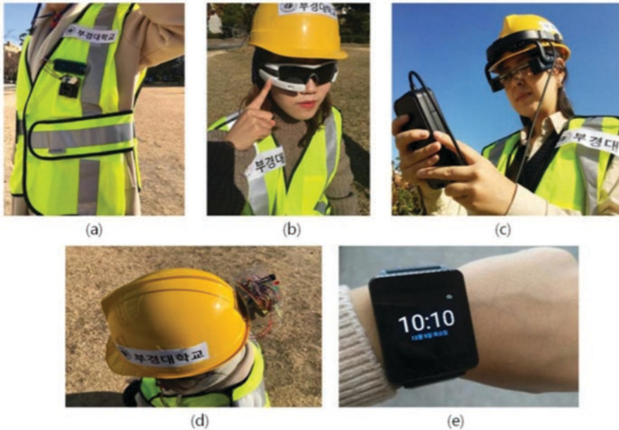
Fig. 3 Different wearables used in the mining industry. (a) Safety vest equipped with sensor, (b) and (c) smart eyewear, (d) smart helmet, (e) smartwatch [3]
