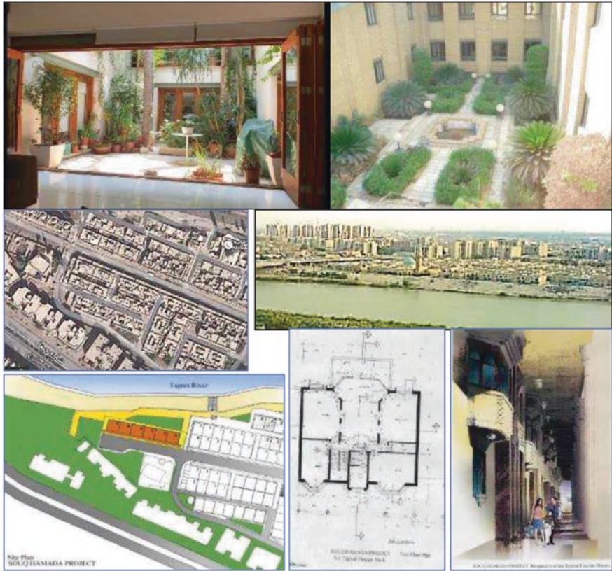
Fig. 9 (Above)—Examples of six row houses close to Tigris River in Baghdad, which use the courtyard design in two floors covered by a dome, and windows from all sides to provide cross ventilation and wind breeze by using traditional materials only. Designed by the author in Baghdad, 1992. (Down)—Souq Hamada neighborhood design by IDRISI Center for Engineering Consultant
