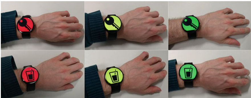
Fig. 13.13 All possible visual feedback modalities presented on the smartwatch. The key symbolizes the lateral grasp and the cup symbolizes the palmar grasp. The color coding conveys the intensity of the FES stimulation, red for high, yellow for medium and green for low
