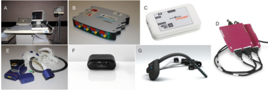
Fig. 3.4 Overview of Amplifiers: (a) old fashioned clinical ink-based EEG device (Neurofax, Nihon Khoden), (b) g.USBamp, 16 channel device, with USB connection to PC (g.tec medical engineering GmbH), (c) 32 channel Liveamp, wireless connection (Brain Products GmbH), (d) ANT Neuro eego amplifier, (e) TMSi water-based EEG, wireless connection, (f) BitBrain Technologies 16 channel brain-amp, wireless connection, (g) unicorn hybrid 8-channel, wireless connection (g.tec medical engineering GmbH)
