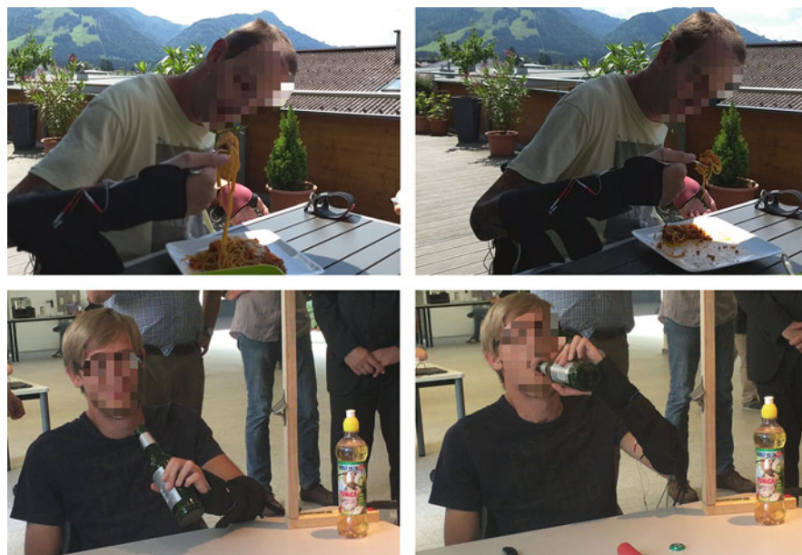
Fig. 13.24 Neuroprosthesis application in daily life settings (Top Row): Participant GRZ003 is using a fork to eat spaghetti. (Bottom Row) Participant UKLHD002 is drinking from a bottle. Both participants use a joystick mounted on the contralateral shoulder to control the MoreGrasp neuroprosthesis
