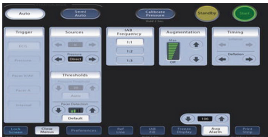
Fig. 27.10 Press “start button,” select mode, and set the frequency at 1:1
