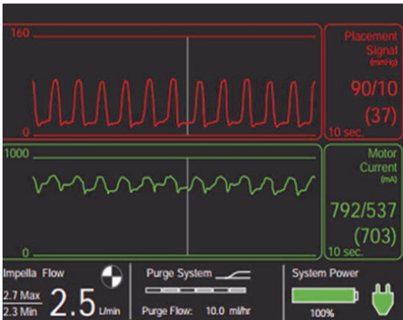
Fig. 27.37 If the Impella advances too far into the LV, the controller will display a ventricular waveform
