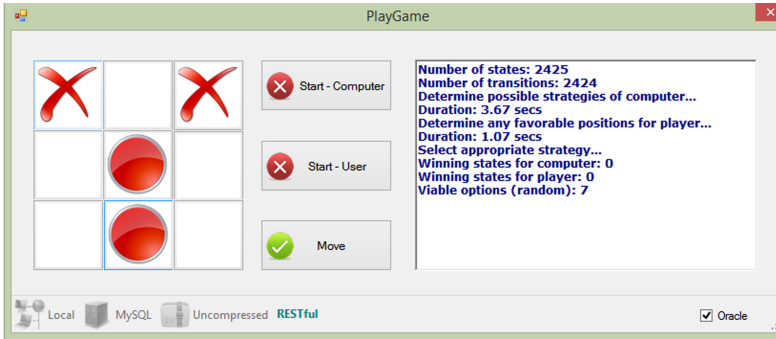
Fig. 6. Use the embedded ATL model checker to determine a winning strategy in Tic-Tac-Toe game
