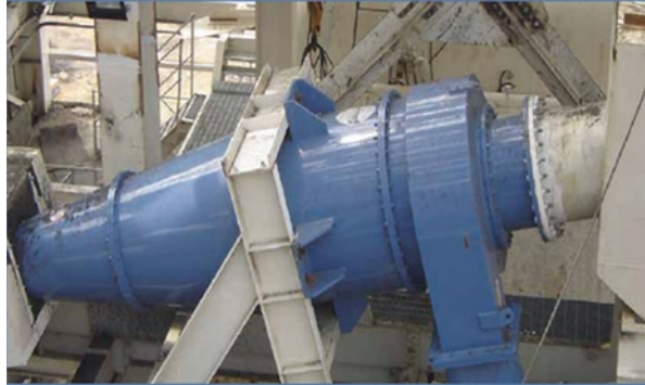
Fig. 1.9 A dense media cyclone (Courtesy: FLSmidth India Limited)
