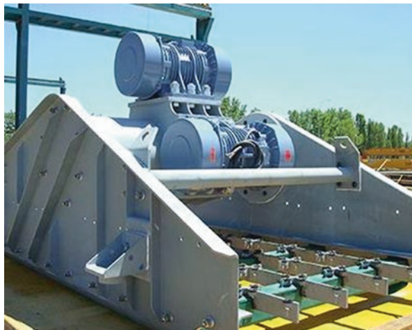
Fig. 1.15 High-frequency dewatering screen (Courtesy: FLSmidth India Limited )
