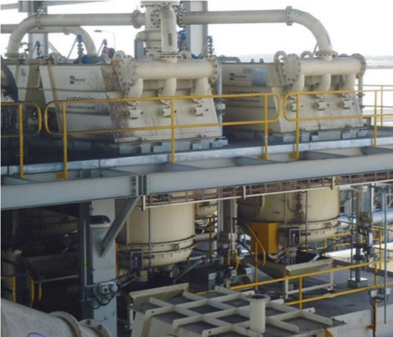
Fig. 1.12 Reflux classifiers (Courtesy: FLSmidth India Limited)
