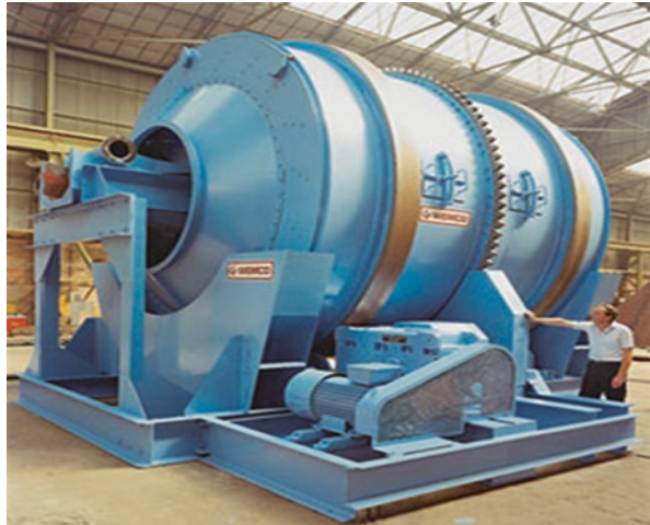
Fig. 1.7 Wemco drum separator (Courtesy: FLSmidth India Limited)
