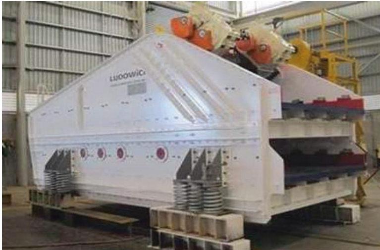
Fig. 1.4 Vibrating screen (Courtesy: FLSmidth India Limited)
