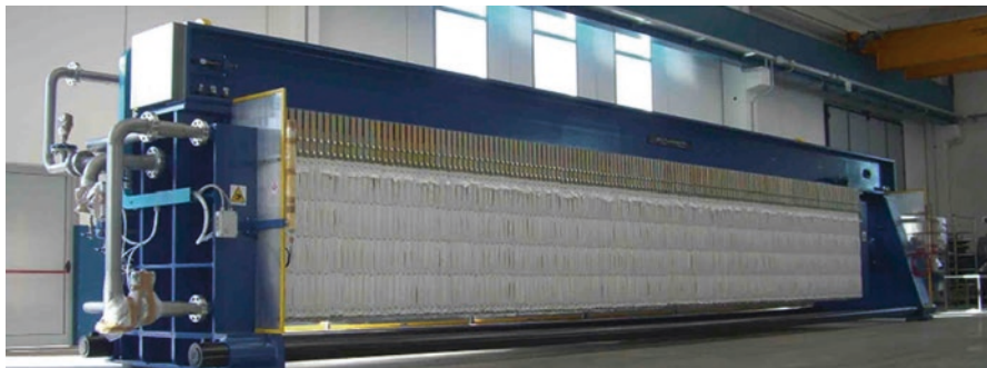
Fig. 1.19 Press filter (Courtesy: Tenova India Private Limited)
