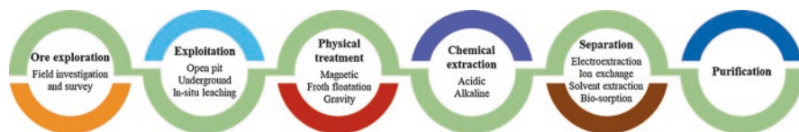
Fig. 16.4 Flow sheet of REE processing from ore minerals
