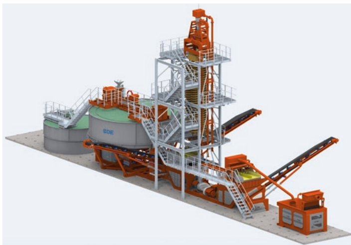
Fig. 1.22 Modular spiral concentrator plant for treating coking coal fines
