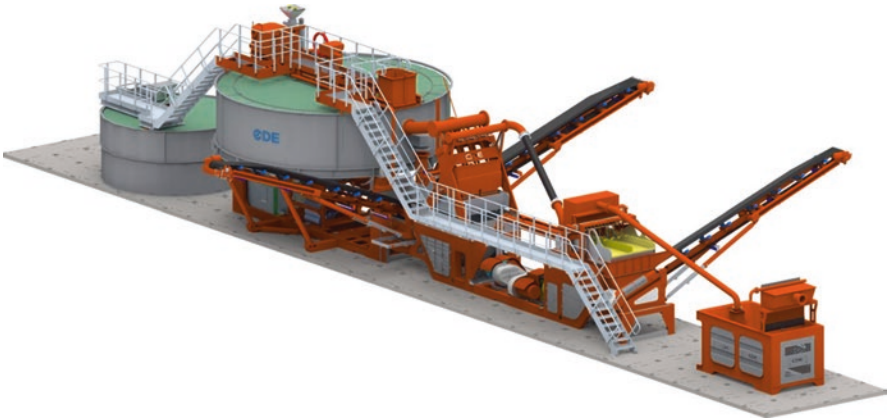
Fig. 1.23 Modular washing plant for treating non-coking coal fines
