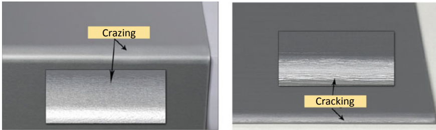
Fig. 2.7 Difference between crazing and cracking ( https://cdn2.hubspot.net/hubfs/3424216/Brochures/White%20Paper_Crazing%20and%20Forming_20180618.pdf )
