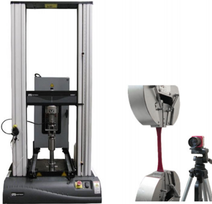
Fig. 11.9 Instron 3367 universal testing and camera testing apparatus
