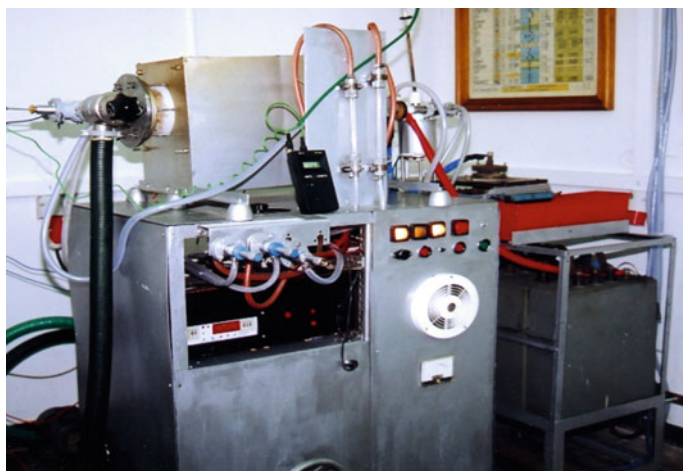
Fig. 13.1 Picture of the plasma-pulse device used for the production of BN coatings
