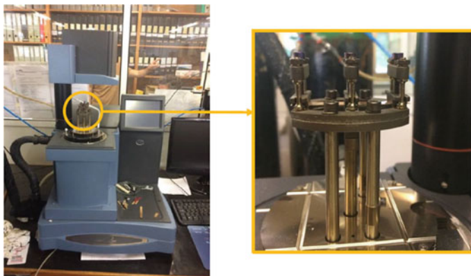
Fig. 8.2 DMA equipment and detail of clamping system
