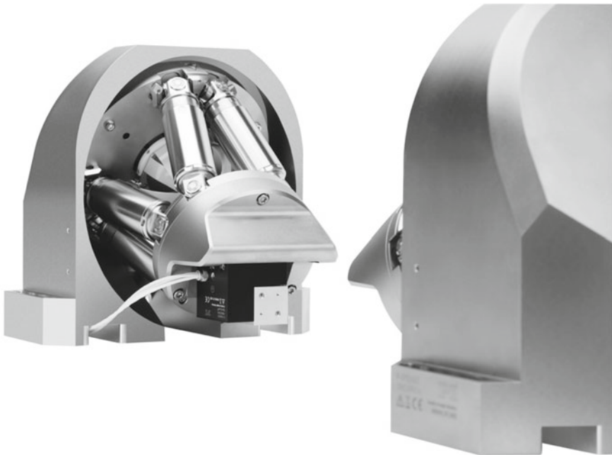
Fig. 9.1 Alignment micro-robots perform multiple alignment processes simultaneously across degrees of freedom, elements, inputs and outputs, even if they optically or geometrically interact
