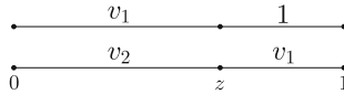
Fig. 1. Strategy for RBS for 2 agents and 2 bikes. The two rows correspond to the behaviour of two agents. Each line segment is labelled with a bike speed that corresponds to the agent travelling on that bike for the distance of the line segment. If an agent walks then the line segment is labelled with 1.
