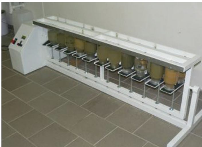
Fig. 7 General aspect of the mechanical shaker device
