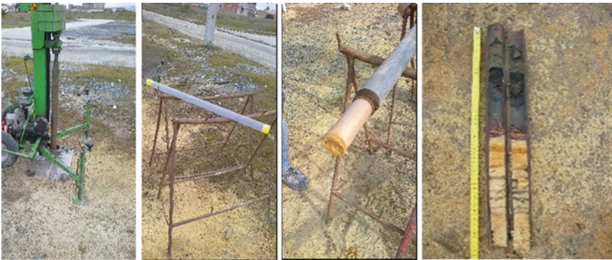
Fig. 6 Different phases during the sampling process using the direct push soil sampling procedure
