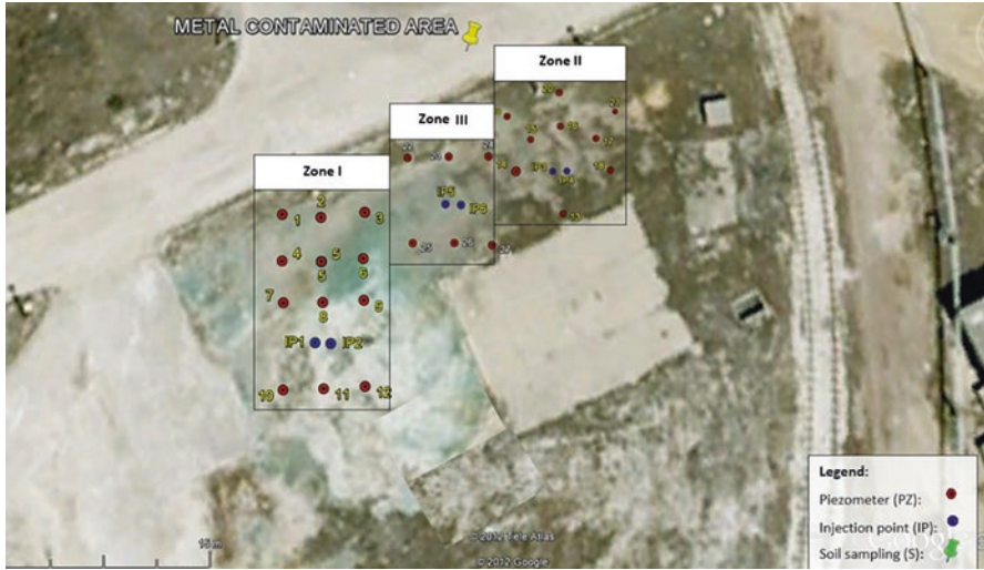
Fig. 12 General aspect of the field testing area, and monitoring point’s distribution for the three zones
