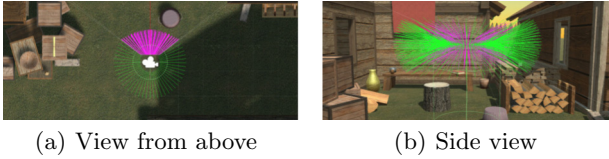
Fig. 12. Third-person example of 360 peripheral: forward-facing rays (magenta), backward-facing rays (green). (Color figure online)
