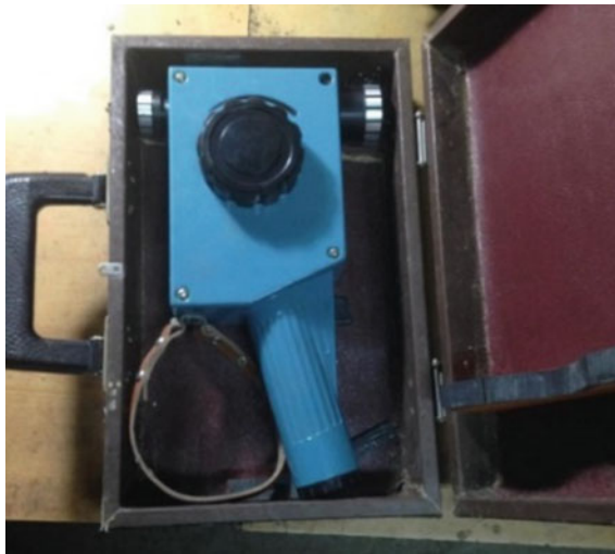
Fig. 7 Disappearing-filament optical pyrometer
