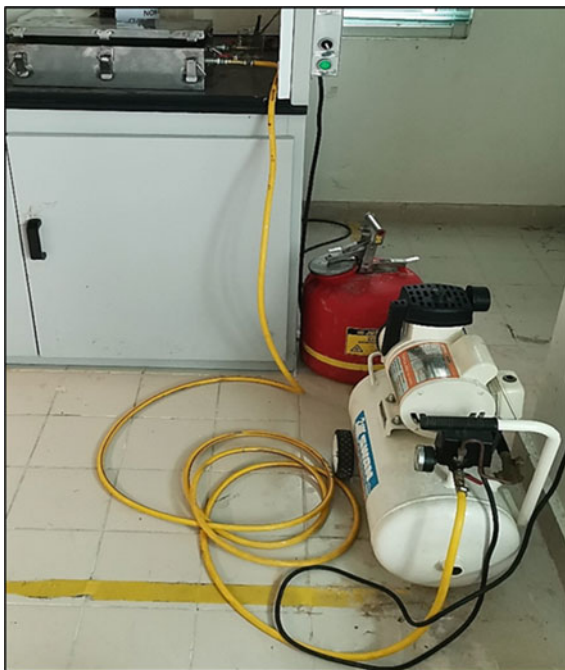
Fig. 4 Vacuum impregnator connected to an air compressor
