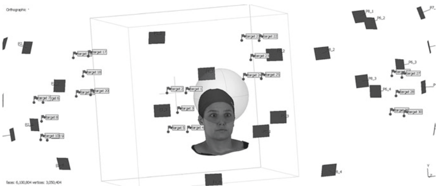
Fig. 3 A CG face generated through photogrammetry using 33 photos captured from different angles
