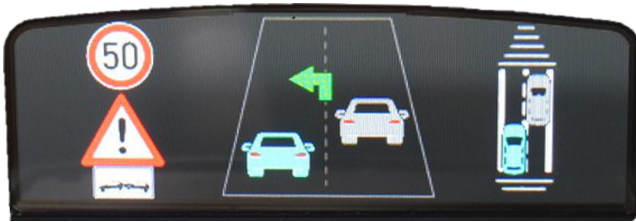
Fig. 9. HMI for cooperative lane change maneuver presented on a combiner HUD (i.e., a HUD, which uses a small plastic screen instead of the windshield to project the information) by Noritel.
