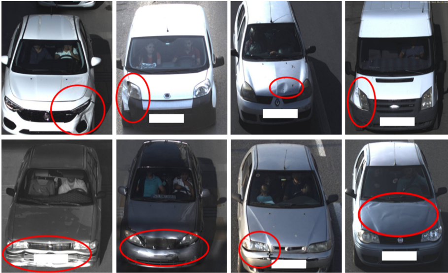
Fig. 2. Damaged vehicle images captured by a roadway surveillance camera. Red rectangles encapsulate the damaged regions.
