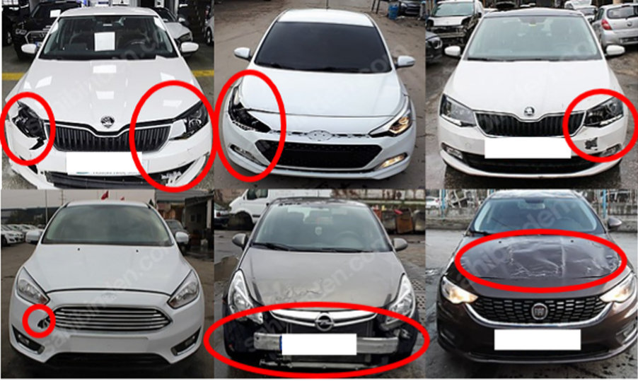
Fig. 14. Sample damaged vehicle images in the test set collected from the Internet [28] with red ellipses enclosing the ground truth damaged areas. The first row shows samples successfully classified as damaged. The second row shows incorrectly classified damaged vehicle samples.
