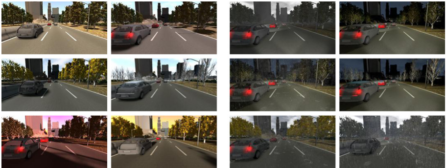
Fig. 3. Samples from the SYNTHIA dataset. All images show the same frame of a driving sequence, but under different environmental and lighting conditions. The two left columns show variations of sunny environments, while the two right columns depict settings with low illumination and adverse weather conditions.
