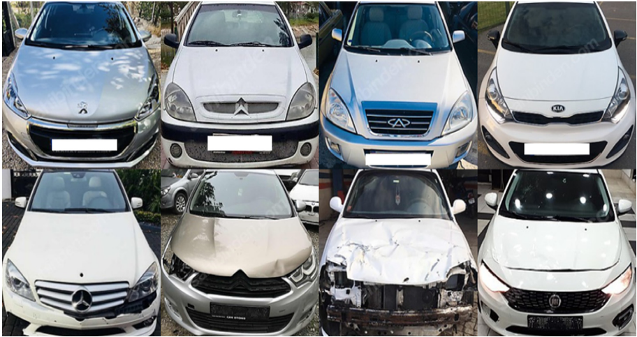
Fig. 11. Sample detected vehicle images from the dataset. The first row shows non-damaged vehicles, the second row shows damaged vehicles.
