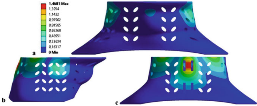
Fig. 14 Deformation (displacement) along the model: a front, b left-side, and c back views [32]
