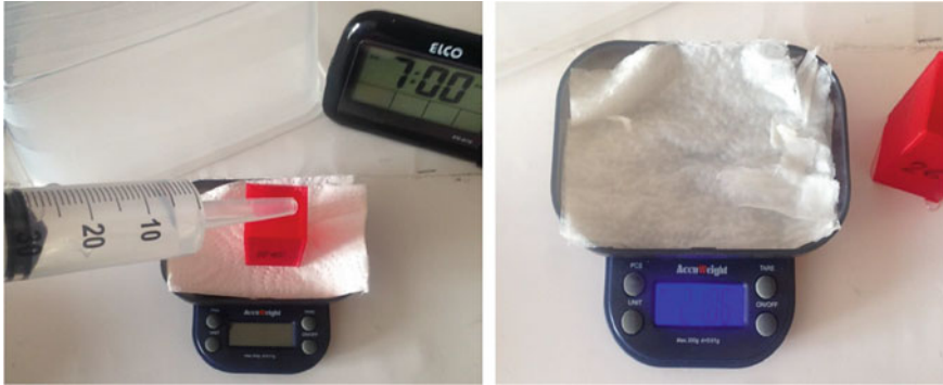
Fig. 3 Tightness test: the digital scale with the absorbent paper sheet is set to zero, the vessel is filled with 30 ml of water and the stopwatch is activated (left); after 7 h, the weight of the amount of water that has leaked and been absorbed by the paper is determined (right)
