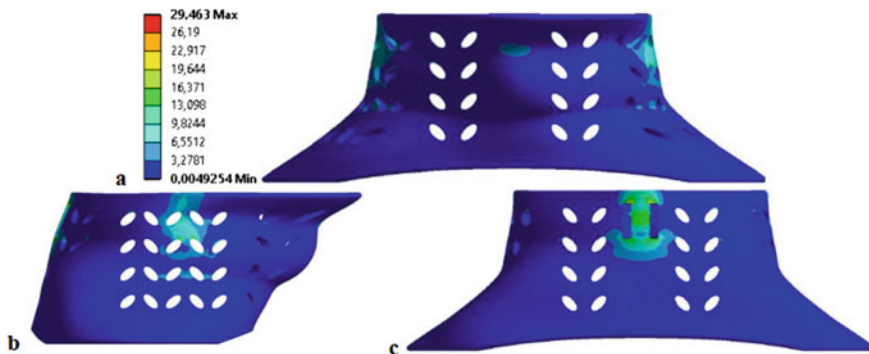
Fig. 13 Stress distribution along the model: a front, b left-side, and c back views [32]
