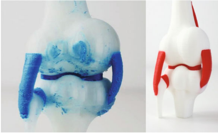
Fig. 10 Knee joint manufactured with two materials, with and without oozing effect: 3D printer with two non-independent extruders (left) 3D printer with independent double extruder–IDEX–(right) [9]
