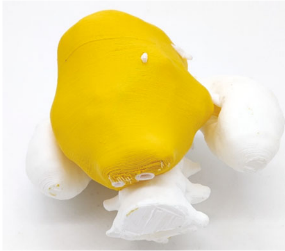
Fig. 7 Example of an FFF training model with the anatomical structures printed in white and the tumour in yellow
