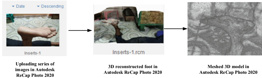
Fig. 7 Proposed approach for image based 3D virtual reconstruction
