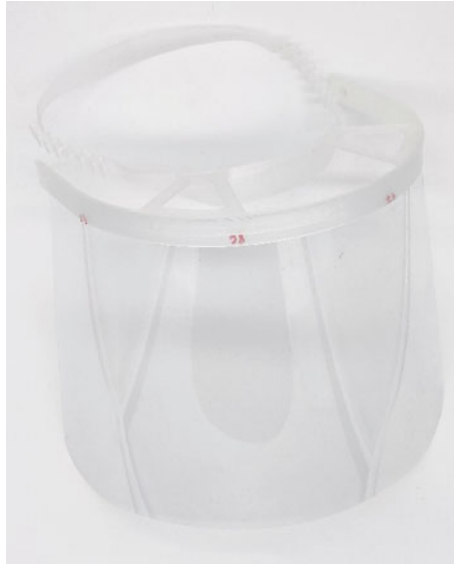
Fig. 14 Face shield 3D printed using FFF. The visor is 3D printed using PP (PolyPropylene) and the screen material is PVC (PolyVinyl Chloride), not 3D printed
