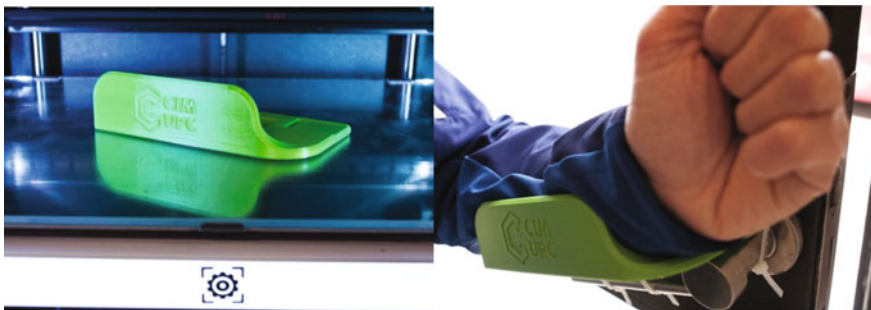
Fig. 13 CIM UPC design of a door opener to fight the spread of Covid-19: 3D printed sample (left) and its use (right)
