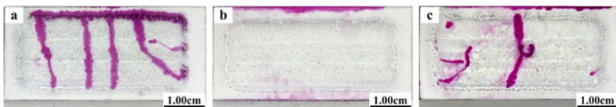
Fig. 2 Cracks morphology of clad layers with different amount of Y_2O_3 . a 0.0 wt%, b 0.3 wt%, c 0.6 wt%
