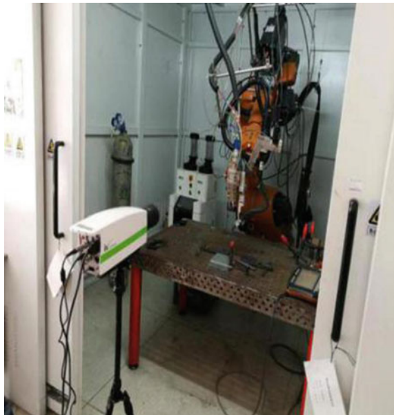
Fig. 1 RC-YLS-2000 fiber laser and manipulator
