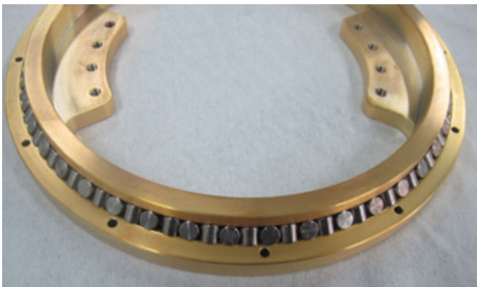
Fig. 2 Four point contact ring structure
