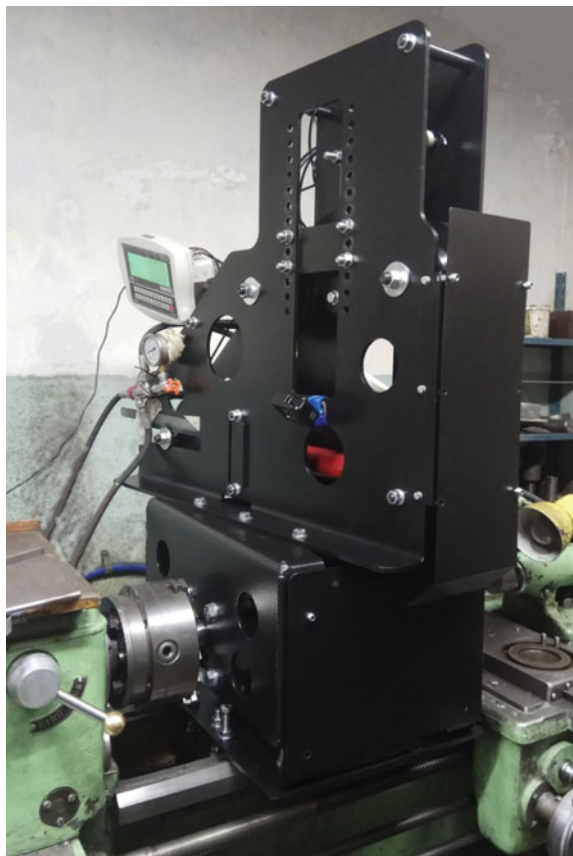
Fig. 12 The wire rope bending stiffness defining scheme
