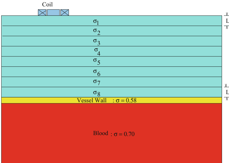
Fig. 10.5 The eight-layer inversion algorithm. The objective is to determine \sigma_1, \dots, \sigma_8 , given that the resolution of the algorithm L = 0.2125 mm
