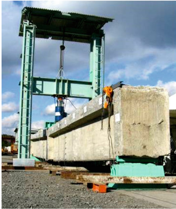
Fig. 6 Loading device for a bending test of the girder
