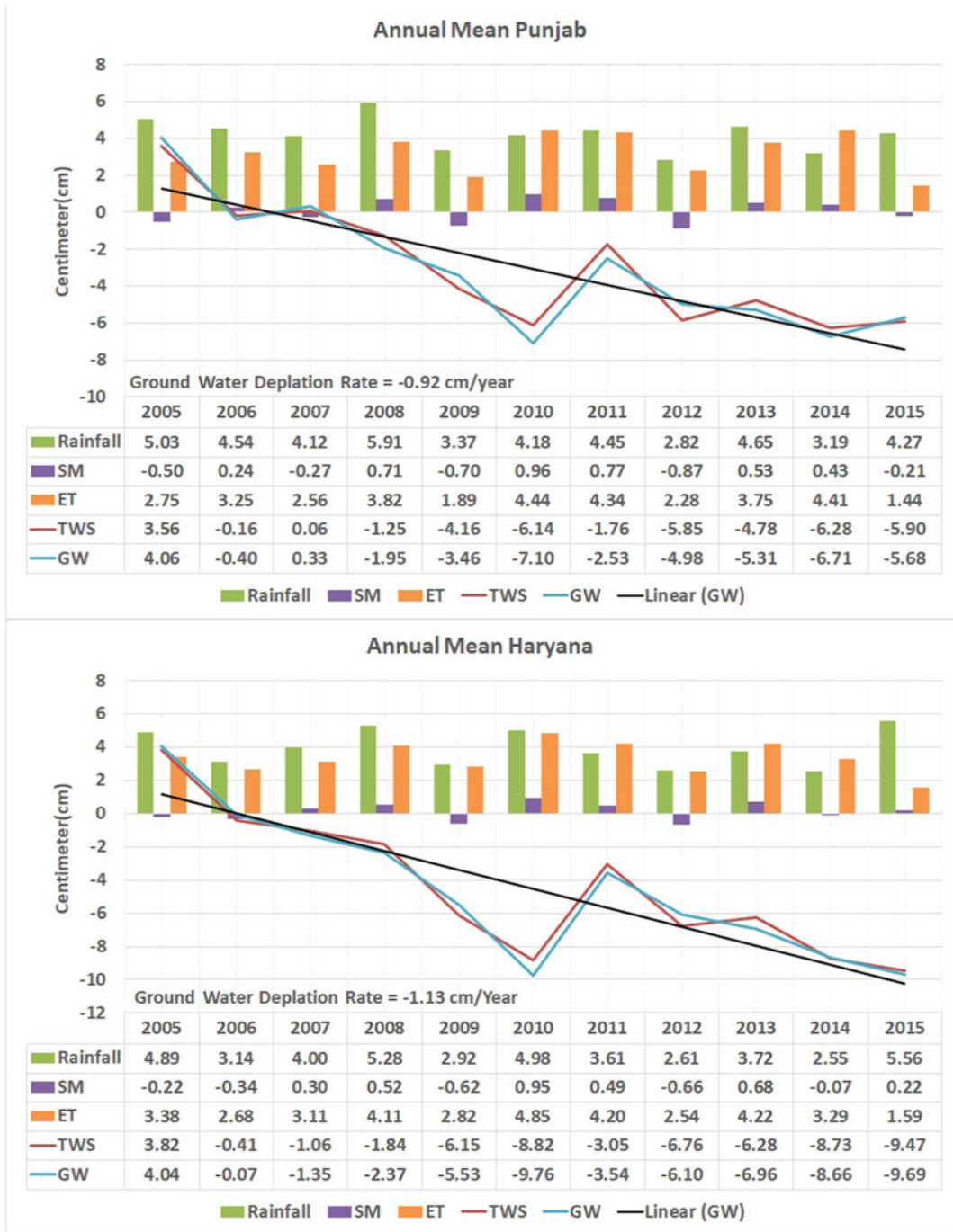
Fig. 11.3 Annual mean groundwater depletions observed by satellite over Punjab and Haryana (Source GRACE data)
