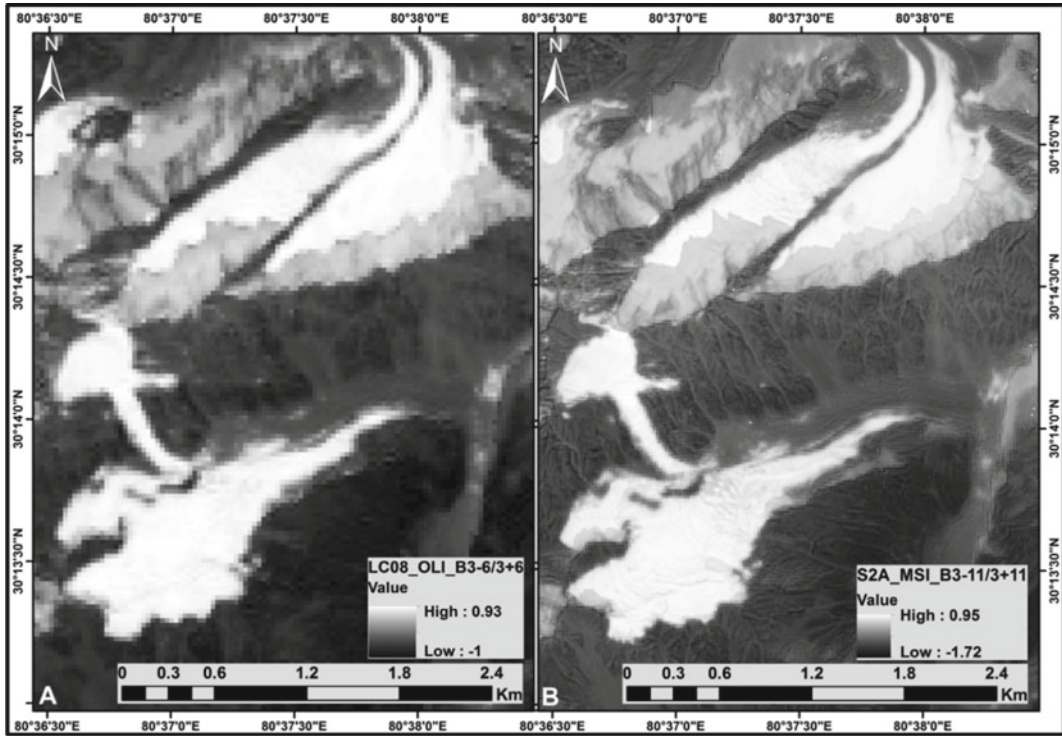
Fig. 4.15 NDSI images: a Landsat OLI (band 3-band 6), b Sentinel-2A MSI (band 3-band 11) (Source WRD-IIR)
