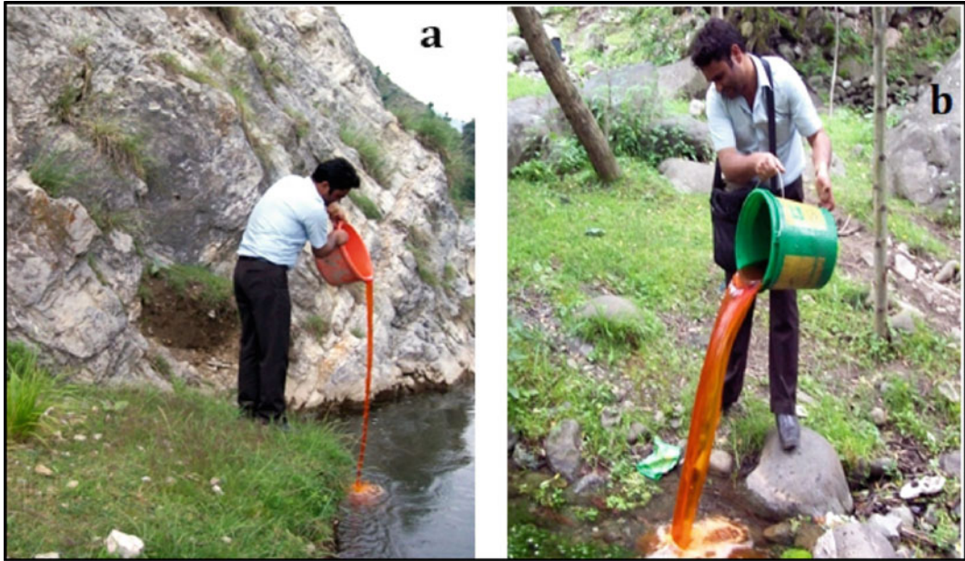
Fig. 20.16 Dye testing carried out near a Adigam and b Gadol confirming connection between recharge sites and Karst springs (Source Authors)
