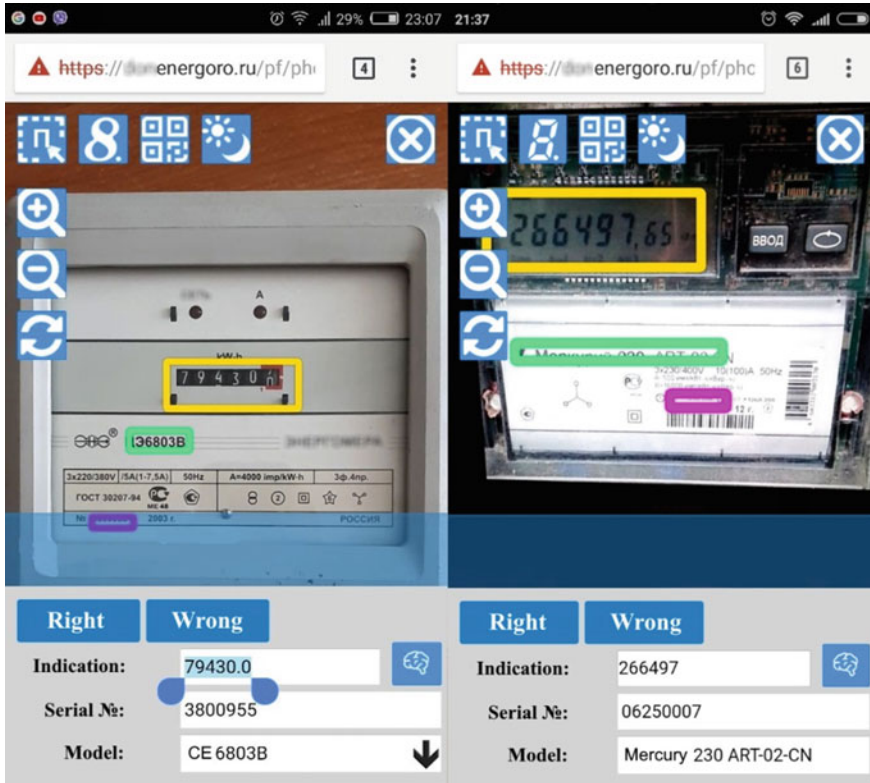
Fig. 4 Examples of meters reading recognition
