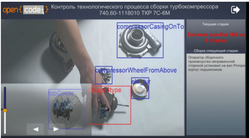
Fig. 3 AR-based intelligent manual operations' control
