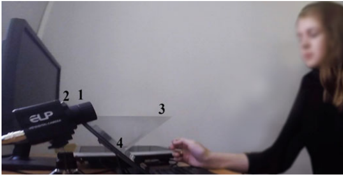
Fig. 3 General view of the information and measuring system of “deep” testing. Legend: 1—digital camera; 2—infrared searchlight; 3—3D-display; 4—laptop with a test program. The photo was taken at real field studies. Some parts of the image are veiled to maintain privacy. A feature of the installation is its hardware availability and high measurement efficiency. Setting the viewing angles (this is important) of web cameras and its adjustment can be done remotely (remotely) using the developed software
