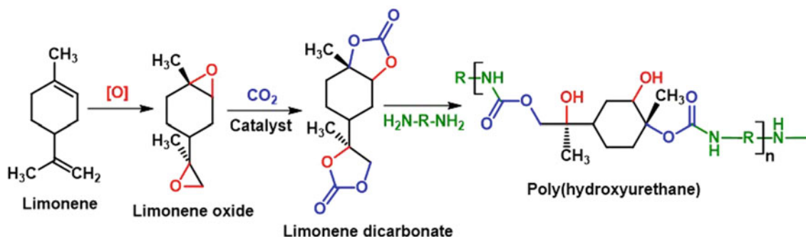
Fig. 22 Synthesis of a limonene oxide-based polyurethane through isocyanate-free polymerization. Adapted with permission from Bähr et al. (2012). Copyright (2012) The Royal Society of Chemistry
