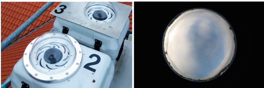
Fig. 1 All-sky images. Left: camera on the rooftop making constant all-sky images (© Philipp Otto); right: one instance of the resulting sequence of images (© Institute for Meteorology and Climatology, Leibniz Universität Hannover)
