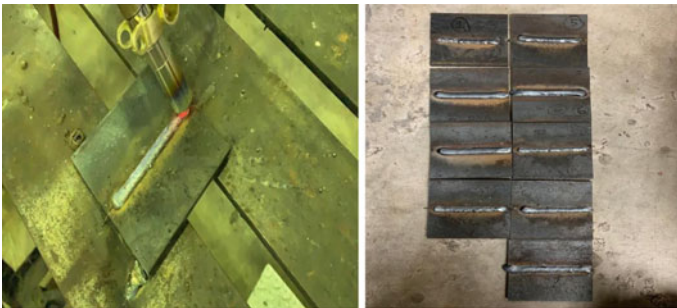
Fig. 22.2 Welding process and welding specimen
