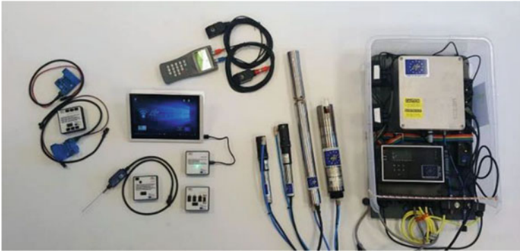
Fig. 2 Elements included in the monitoring Kit (Plug&Glean)
