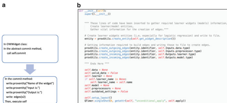
Fig. 3.4 Provenance capture instrumentation via the Orange3 GUI. (a) Diagrammatic overview of GUI-based capture. (b) Example code required to add provenance capture to Orange widgets
